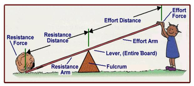
A lever either uses less force over a greater distance or more force over a shorter distance.
