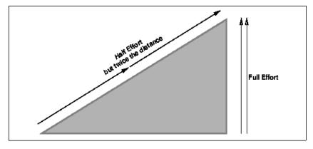
An inclined plane allows for less force over a greater distance.
