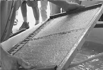
Next, the pulp was put on a special mold called a deckle. The deckle gave paper its flat shape.
