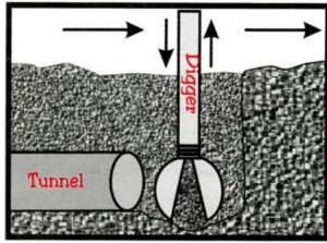
The first tunnel finished in the Big Dig doesn't go under the city. It goes under Boston Harbor. Workers used the "sunken tube" method. A big ditch was dug in the ground under the water with dredging machines. Tunnel tubes with caps on the ends were pre-made on land and floated over on barges. The tubes were placed under water in the ditch. The caps kept water out. Divers attached the tubes together. The caps were then removed and the tubes were covered with soil.
