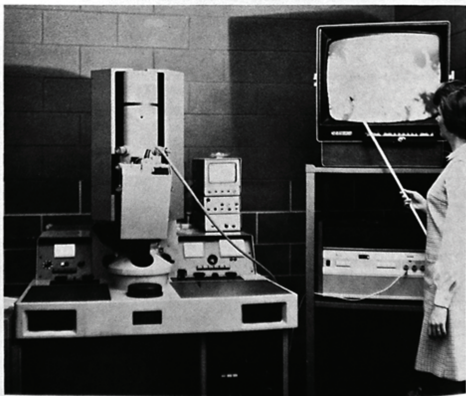
The Weatherscope at right displays pictures received from American weather satellites. It was donated by Scientific Atlanta. The Carl Zeiss EM9 electron microscope at left can magnify up to 400,000 times, and is employed for both instruction and research. Several Zeiss optical microscopes are also in use at Fernbank, including one for photomicrography.
