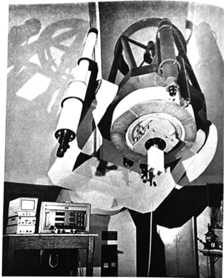
The principal astronomical apparatus at Fernbank Science Center are a Carl Zeiss Mark V planetarium projector (at left) and a Tinsley 36-inch Ritchey-Chretien reflector. Seventeen feet long, the Mark V contains 153 single and double projection lenses. The Zeiss sky scene above includes the moon, part of the Teapot in Sagittarius, and the globular cluster M22. Kirby Freeman's photograph of the 36-inch shows finder and guide instruments, as well as the solar prominence telescope that is mounted on the left arm of the fork.
